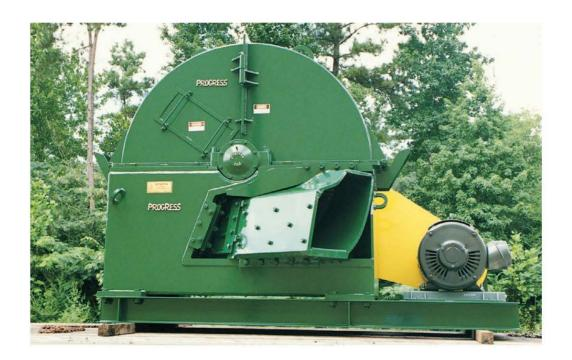
The chipper is available in 4,6 or 8 knives for chip lengths 1/2" to 1", to meet customer's requirements. Discharges are also available in top, bottom, side and back arrangement.
