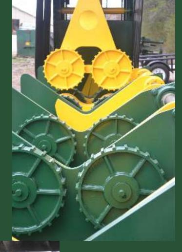
The frame of the cutter unit carries the hold-down arm and the movable cutter. The cutter is placed below the V-block level and powered by an electric motor via a coupling. The cutter head is made in replaceable segments. Knives are four(4) sided for turnable usage.
