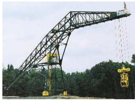
Log crane sizes range from 75' to 175' with 14 to 45 ton gross capacity.
